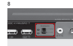
8 Console selection : T only : only console in transmitter can be operated T+R : consoles in both transmitter and receiver can be operated
