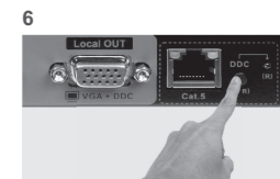
6 Set DDC in transmitter : Red LED on : DDC in receiver is stored Red LED off : DDC in transmitter is stored
