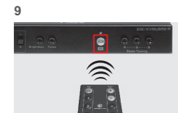
9 If necessary ; use I.R remote controller to fine tune R.G.B skew
