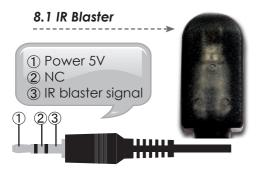
**Note:** The frequency on both IR Receiver & Blaster can support 36~387KHz with NEC code.
